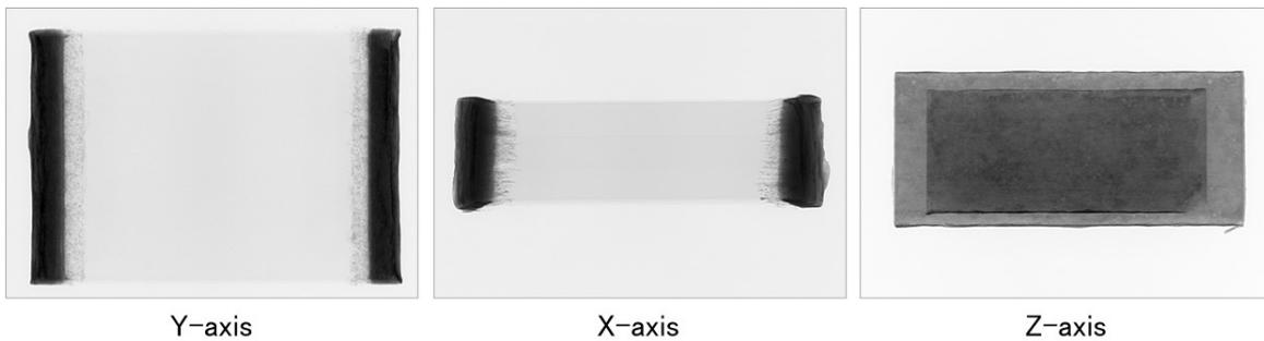
Fig. 11. The result of radiographic examination of stacked metallized film chip capacitor
