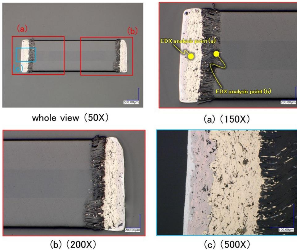
Fig. 12. The result of cross-section observation of stacked metallized film chip capacitor
