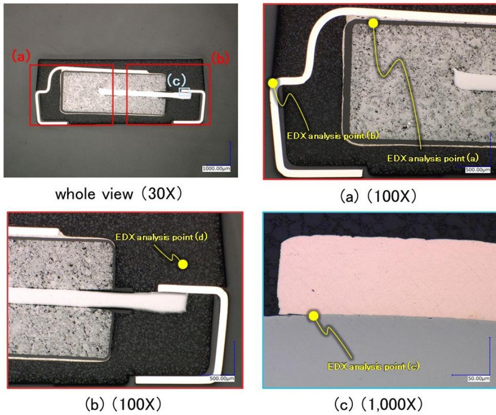
Fig. 4. The result of cross-section observation of polymer tantalum capacitor
