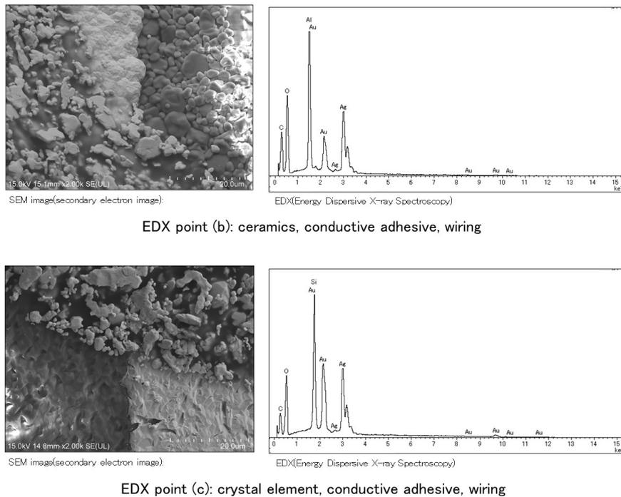
Fig. 17. The result of SEM / EDX analysis of voltage-controlled crystal oscillator
