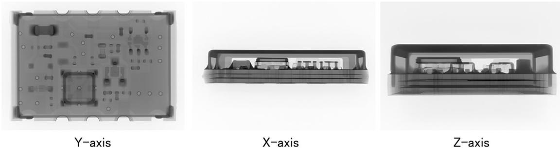
Fig. 15. The result of radiographic examination of voltage-controlled crystal oscillator
