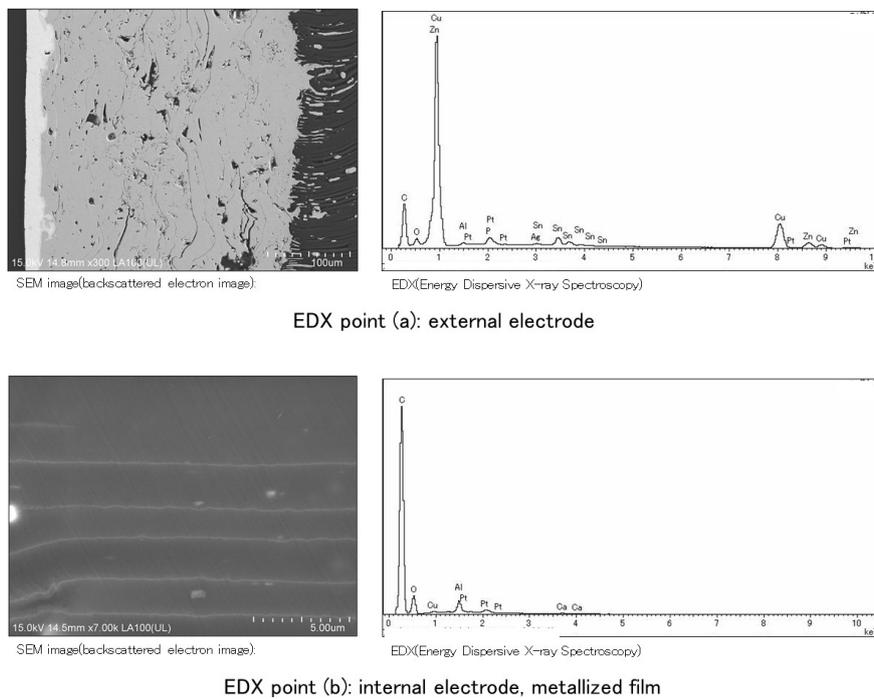
Fig. 13. The result of SEM / EDX analysis of stacked metallized film chip capacitor
