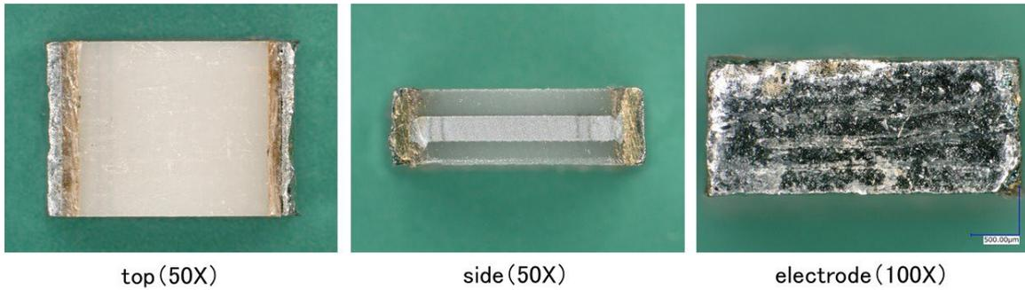
Fig. 10. The result of the external visual examination of stacked metallized film chip capacitor
