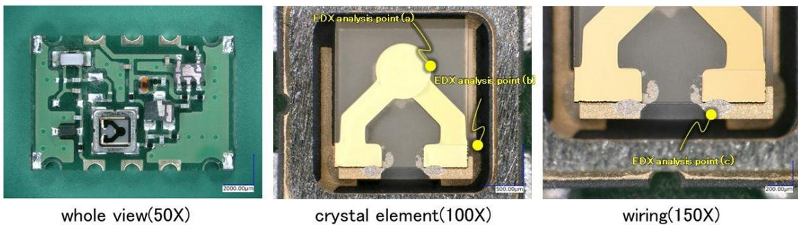
Fig. 16. The result of the internal visual examination of voltage-controlled crystal oscillator
