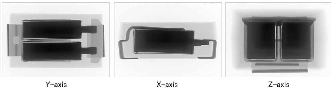
Fig. 3. The result of radiographic examination of polymer tantalum capacitor
