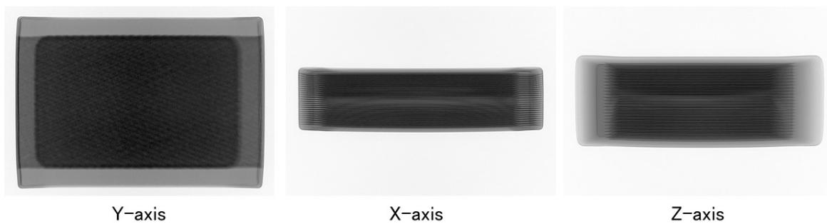
Fig. 7. The result of radiographic examination of solid state battery
