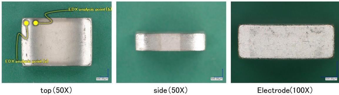
Fig. 6. The result of the external visual examination of solid state battery
