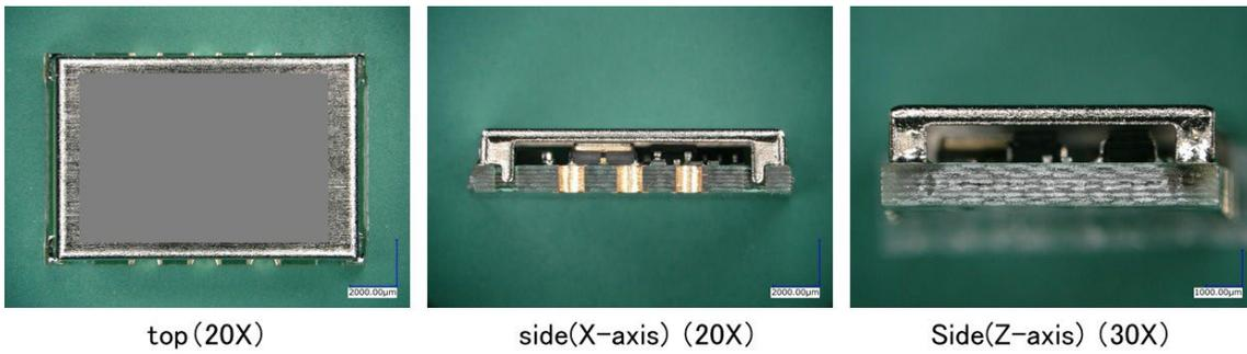
Fig. 14. The result of the external visual examination of voltage-controlled crystal oscillator
