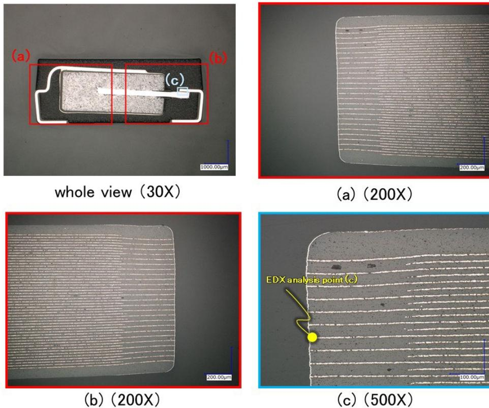
Fig. 8. The result of cross-section observation of solid state battery
